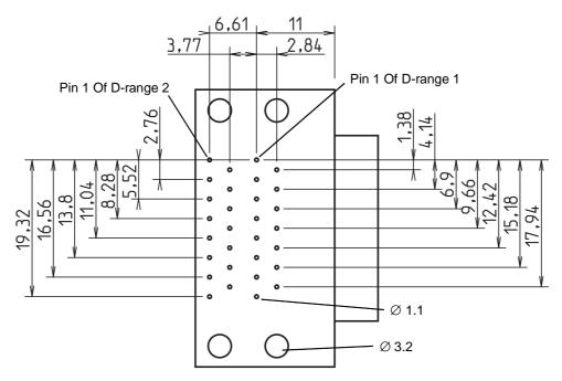
Figure 5 D-range Connector Dimensions
