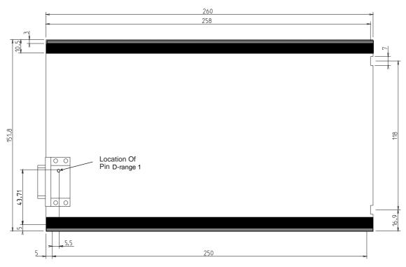
Figure 4 Main PCB Dimensions
