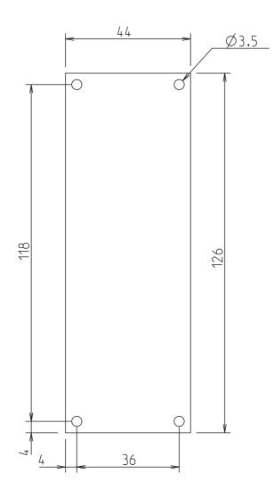
Figure 6 Front Panel PCB Dimensions
