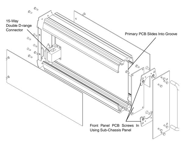
Figure 7 T800-08-0000 Ancillary Module Chassis
