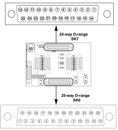
Figure 3 T800-50-0000 Backplane PCB Showing D-range Location
