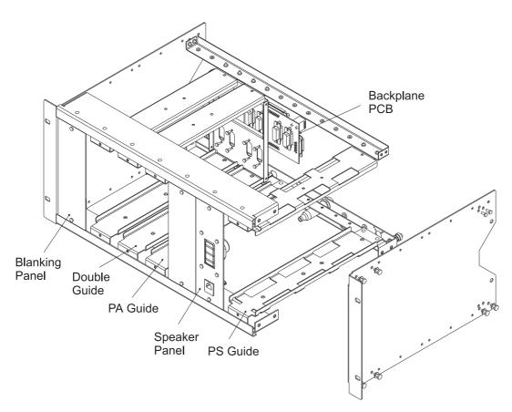
Figure 1 Mechanical Layout Of The T800-22-0000 Rack Frame
